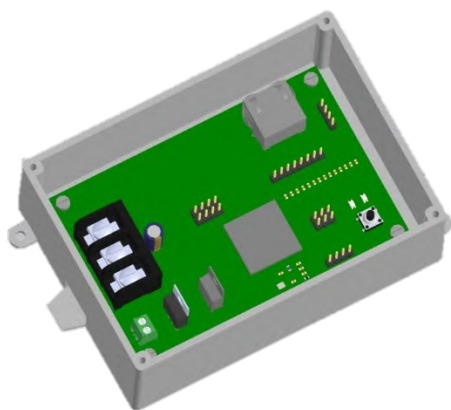
Fig. 4. Computer model of the color control and data processing unit (without cover).
